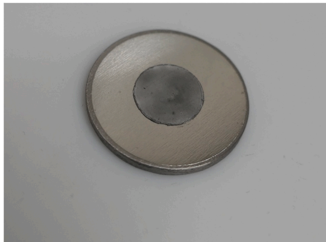
Fig. 5. Photograph of \text{Gd}_2\text{O}_3 targets produced with SPS.
