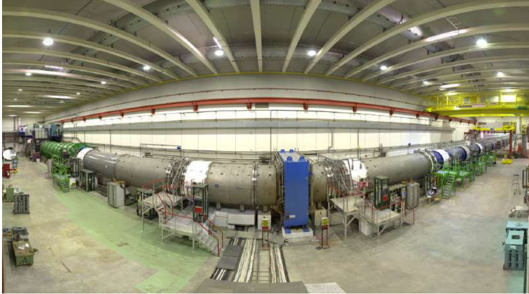
FIGURE 4.2: The ECN3 cavern and the NA62 experiment. The beam enters the cavern from the right. From [182].
