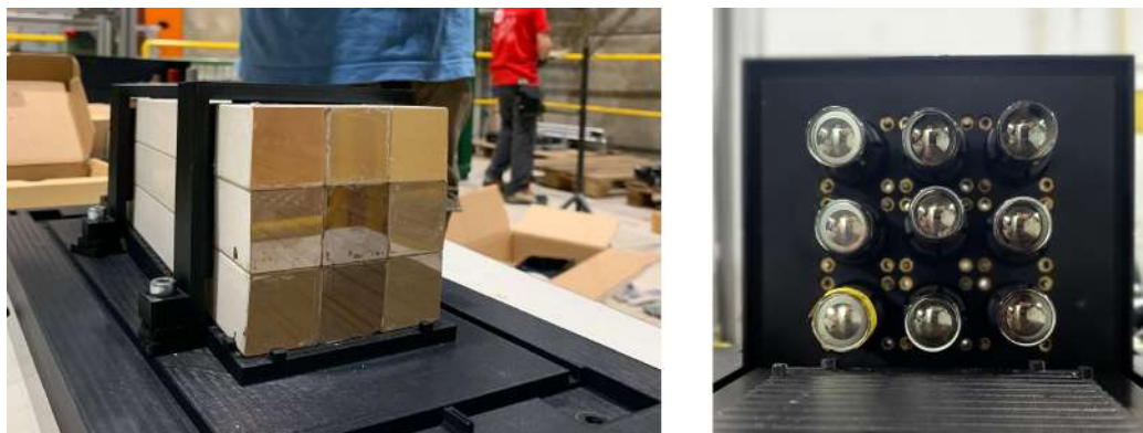
FIGURE 2.13: The Genni calorimeter: pictures of ( left ) the crystal matrix and ( right ) the PMT matrix.
