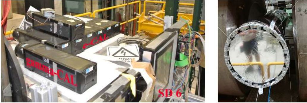
FIGURE 2.21: Downstream stage of the KLEVER 2018 beamtest: ( left ) calorimeters and SD6 tracking module, and ( right ) rear side of the helium bag.
