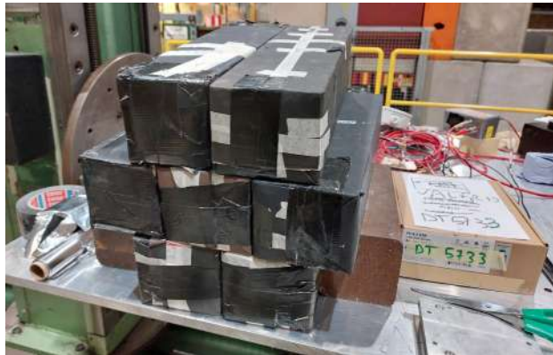
FIGURE 2.24: Hibiscus-like array of lead glass blocks used as electromagnetic calorimeter in the STORM 2022 beamtest on CERN H2.
