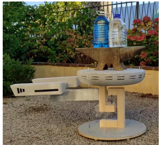
Fig. 3.8: Tensegrity table to study forces: https://www.youtube.com/watch?v=fxMhk4_Ploo
