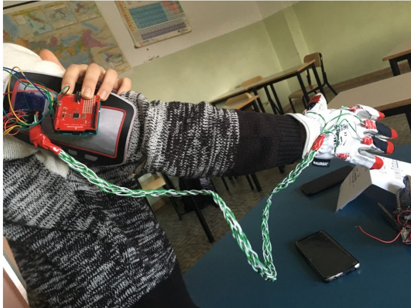
Fig. 3.10: Musical glove: a glove with sensors, which plays music when the fingers bend (designed to promote rehabilitation) https://www.youtube.com/watch?v=ZWut7Ps-4mE
