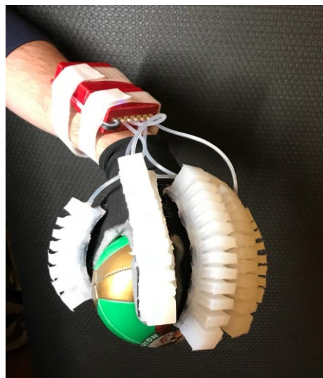
Fig. 3.9: Softrobotic glove: a glove with softrobotic actuators controlled by an air pump, capable of helping to open and close a hand https://youtu.be/1JPcmn5rvNY
