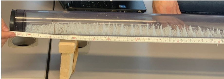
Fig. 3.7: Kundt 's tube to study sound waves https://www.youtube.com/watch?v=bqGSOT3Gllc
