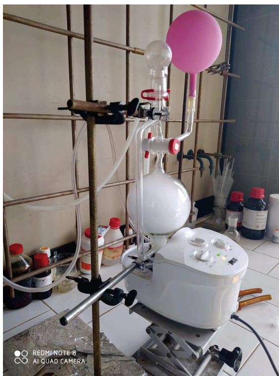
Figure 12: Picture of the batch aerosol reactor during a reaction.
