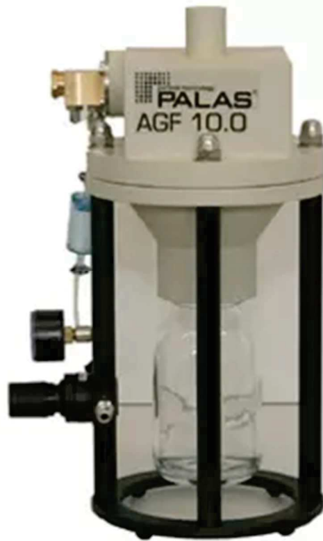
Figure 4: Commercially available Laskin nebulizer.
