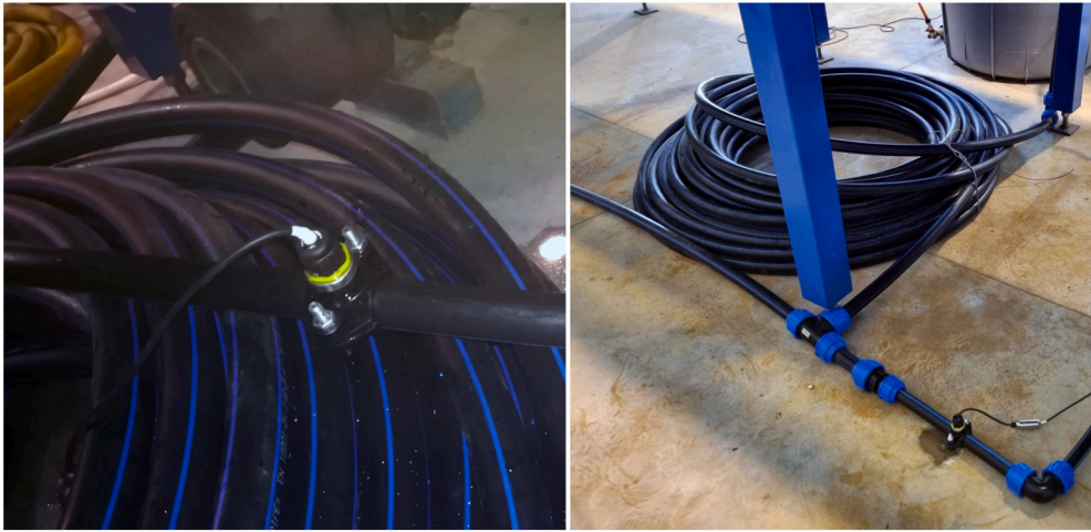
Fig. 2. Pictures of the two hydrophone fitted in the pipes of test-rig.
