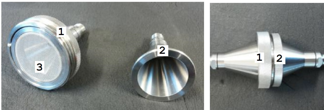
Figure C.1: Filter Holder open (left) and closed (right). The filter is inserted on the metal grid (3) while the metal rings (1) and (2) are screwed in. The external area of the filter is in contact with the metal rings to ensure the sealing. Photo credit Matteo Piazza.
