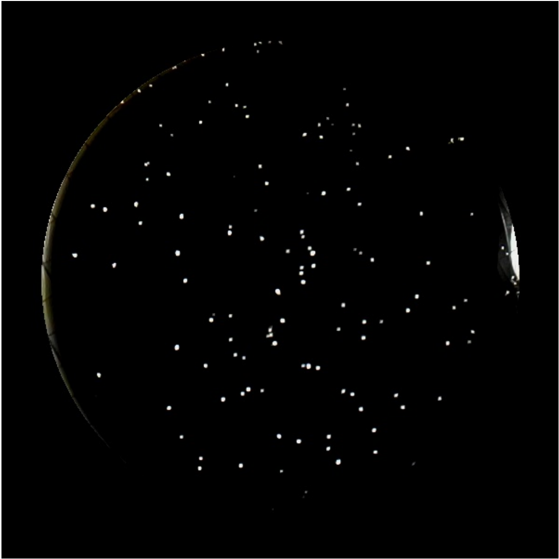
Figure B.2: Figure B.1 after the selection with ImageJ which is used also to center the filter and measure its diameter in pixel units. This picture is saved as 'Image.bmp' in a Matlab folder for subsequent analysis.
