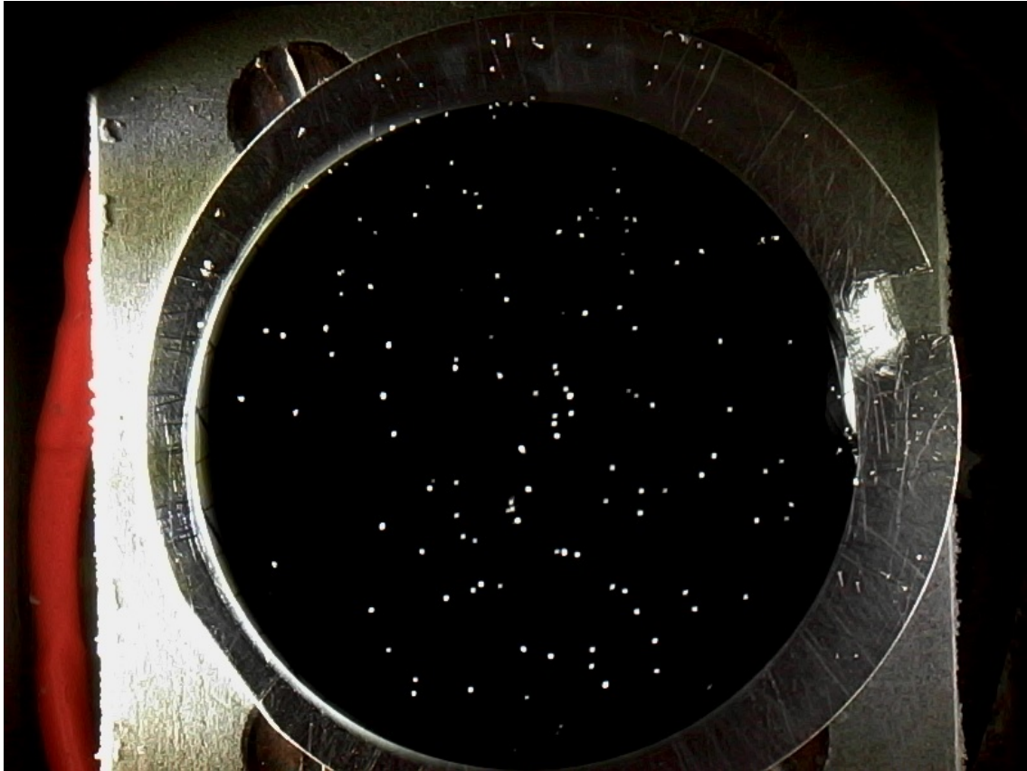
Figure B.1: Picture taken from the usb camera on the PM10 filter from Cimone Montain campaign (sampled on October the 8 th 2015, afternoon) and processed inside the DFPC. Ice crystals are seen as white dots as they reflect the light which is pointed on the filter from a led source fixed at the left of the image. It can be seen that the combined structure filter plus metal plate is placed on the Peltier cooler support.
