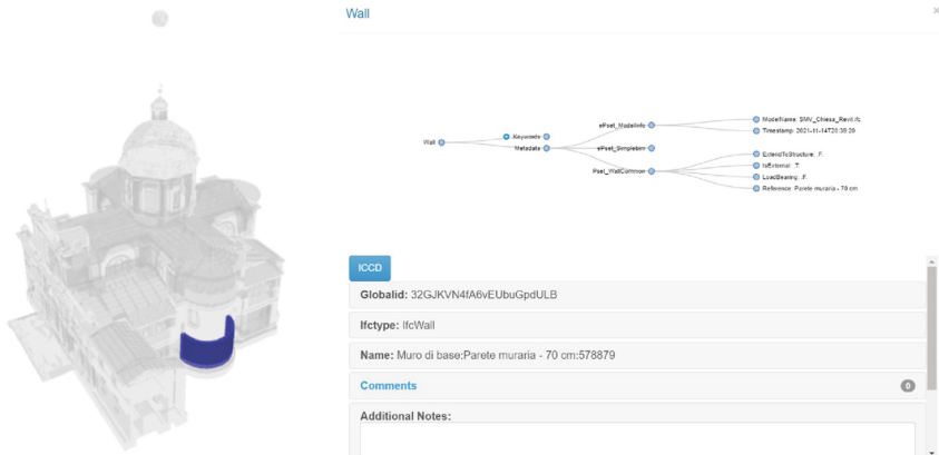
Fig. 3. Every element of the building can be used to perform a live SPARQL query that returns all the details for that element, according to the HBIM ontology. Each value can be updated via web, thanks to the SPARQL 1.1 Update functionalities.
