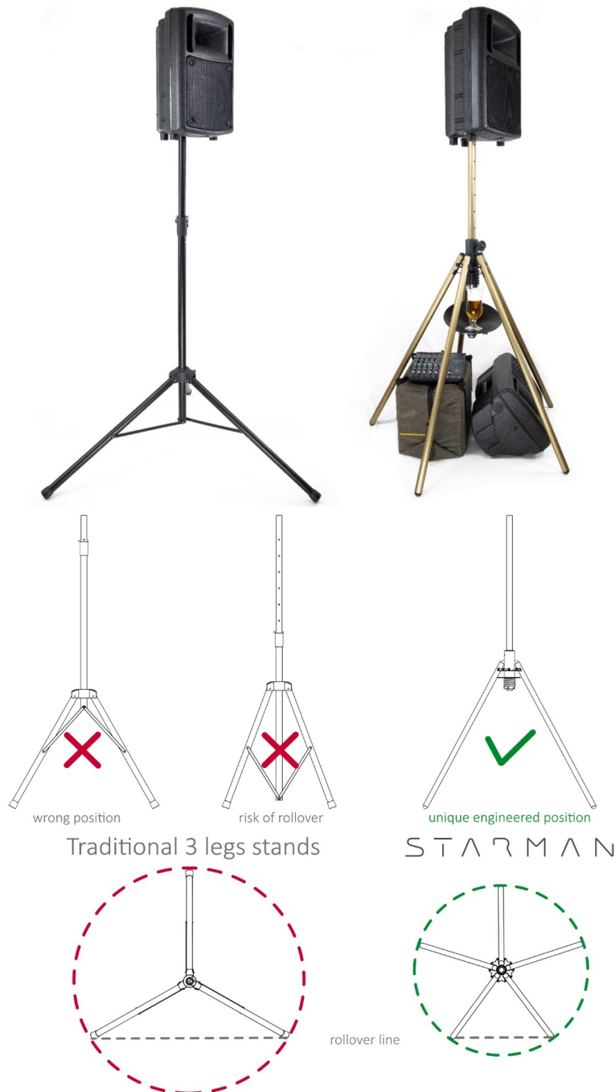
Fig. 1 Traditional speaker stand (left) vs. Starman new stand (right). Designed by Marco Mancini, Courtesy of Starman-stand, Italy. With 5 legs the rollover line is further from the centre of gravity: it is possible to reduce the footprint.
