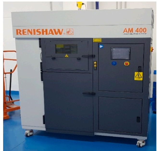
Fig. 1. The 3D printer Renishaw® AM 400 used for printing the components.
