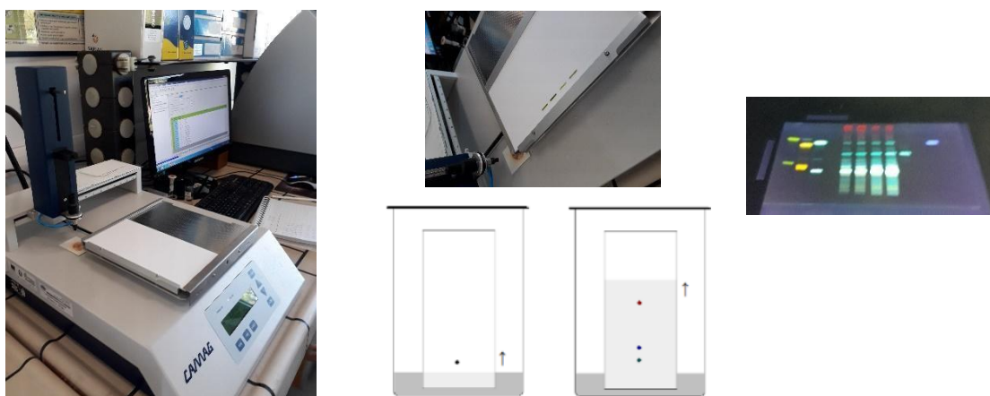
Figure 10. Chromatographic separation in TLC (Pharmaceutical biology laboratories, Malborghetto 2018)
