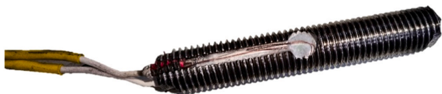
Fig. 13. Stud bolt with strain gauges installed.
