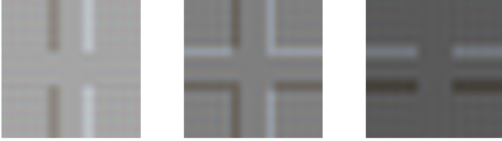
Figure 4.3: DIC images are direction-sensitive. From left to right: cross object computed as in Figure 4.2 acquired at shear angles \tau = 0, \pi/4, \pi/2 rad respectively. According to the direction, the information on one of the two crossing bars might be lost.
