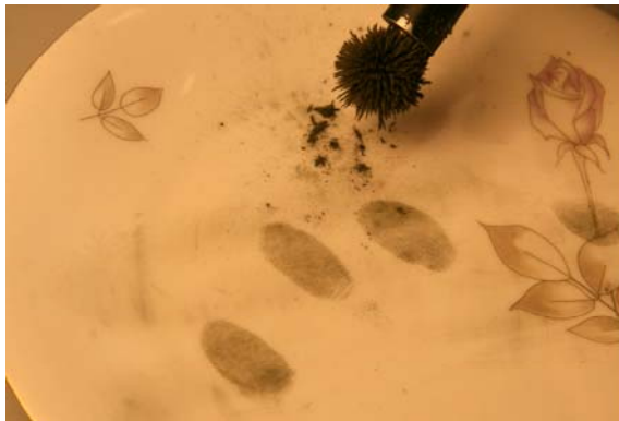
Fig. 15: Fingerprint enhanced with magnetic powder applied by a magnetic brush.
