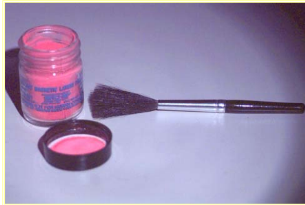
Fig. 14: UV Luminescent powder with a squirrel brush.
